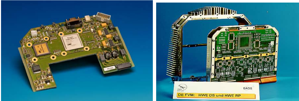
Figure 8: Photograph of a digital waveform generator (left), signal & data processor (right).
